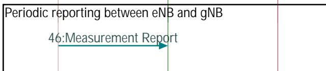
The UE reports measurements to the MN-eNodeB. The measurements include results from 5G NR cells.
